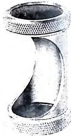
POLAROID — Hand Polariscope, used in the determination of gem stones. All amorphous substances (glass, etc., not under strain), and all isometric gem stones can be easily and quickly separated from those belonging to other crystal systems. See text for detailed description.
